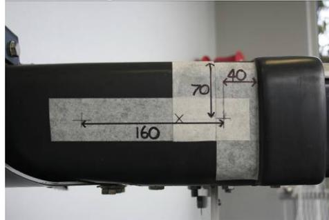
2. Mark bumperette as per photo. Drill two outer holes to 6mm and hole for wiring to 10mm. About 50mm in from screw holes.
