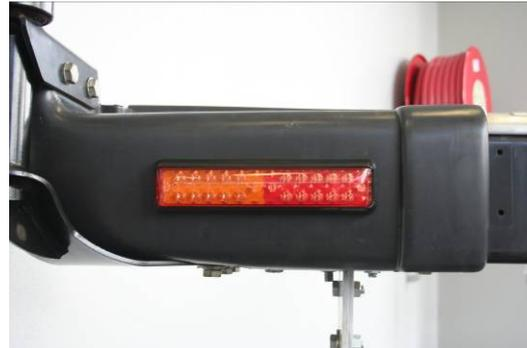
4. Feed wiring through 10mm hole. Clip LED lens back into housing.
